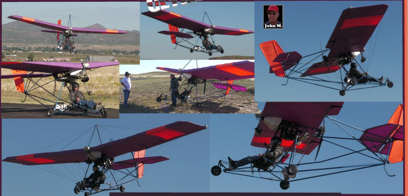
John has been flying ultralights for 15 years. He learned to fly ultralights at Cushing airport in Newark, Illinois. This ultralight plane is a 2004 Quicksilver Sport with conventional 3-axis controls 503 Rotax 2 cycle engine at 53HP. Cruise speed is 50MPH
