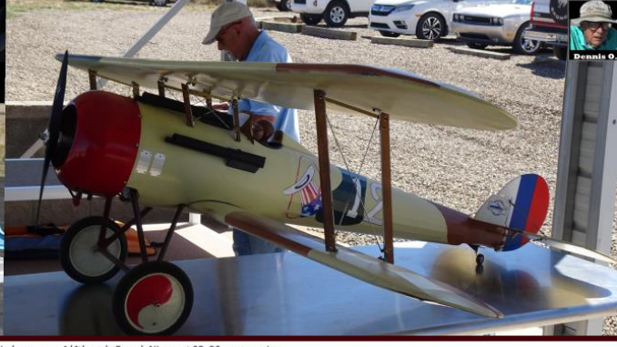
Airplane ..... 1/4th scale French Nieuport 28, 26cc gas engine.
