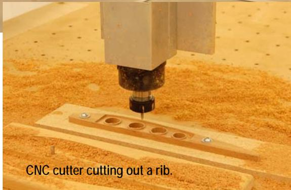
CNC cutter cutting out a rib.
