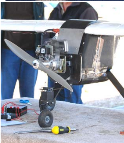
The 28+ pound airplane is powered by a G-62 the club donated to ERAU last year.
