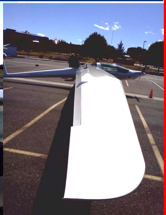
The Eco Eagle is powered by both gas and electric fuel. This innovative design switched in mid flight from gas to electric power in August this year in a flight from Florida campus, an aviation first.
