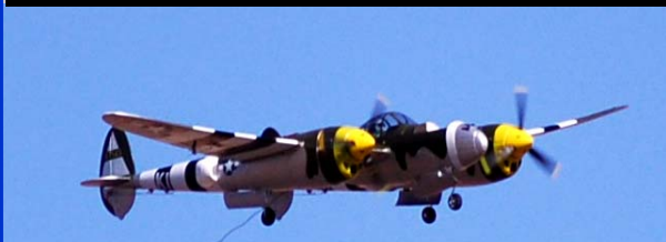
This is a 58" WS foam P-38 sold by Banana Hobby . Motors are two Brushless 1100kv with twin 30 amp ESC's. She flies with one 11.1V 2200mAh Li-Po Battery for power.
