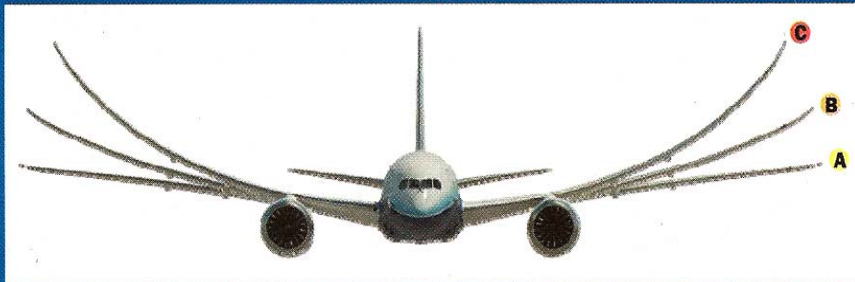
A On ground B 1-g Flight (~12 ft.) C Ultimate load (~26 ft.) Source: Boeing
