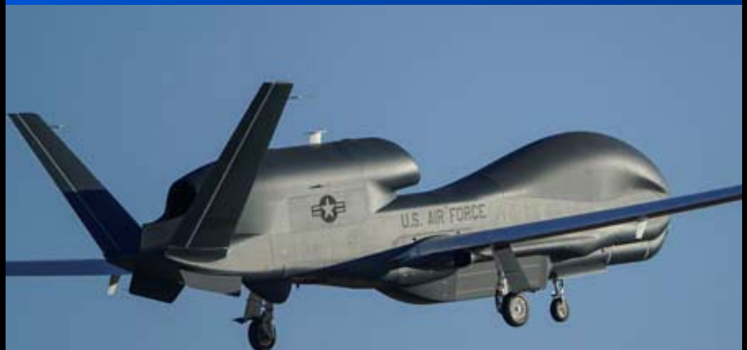
A Northrop Grumman RQ-4 Global Hawk Block 40 remotely piloted aircraft in flight. The Block 40 is one of three variants of the high-flying, long-endurance Global Hawk that the Air Force currently operates. It carries the advanced synthetic aperture radar imaging and tracking for moving ground targets.
