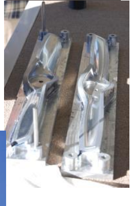
Chuck Heberstreits Glassaire and his prop molds.
