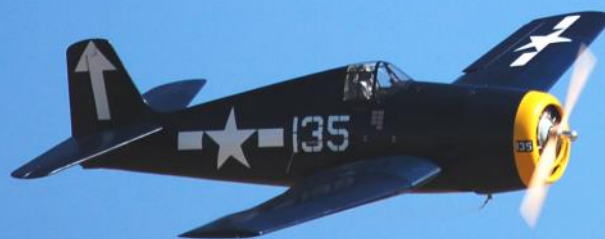
Dennis powers his Hellcat with a 98cc gas engine!
