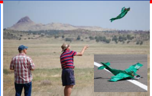
Editor Bob's EP foam dragon, it flew but only for a few seconds, it needs a bigger wing but that's what designing with foam board is all about. A second version will make another appearance before summer's end.
