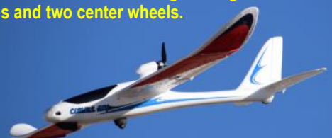
A Don Ferguson sequence with his AXN glider he modified with wing landing skids and two center wheels.
