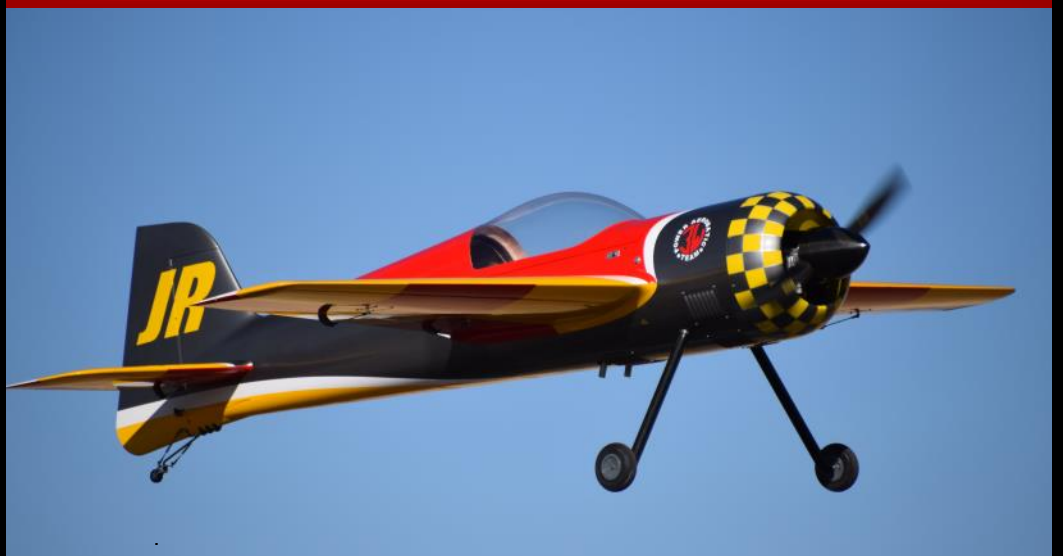
The plane is a 3 meter Composite ARF Yak 55SM with a German 3W 170cc engine. The Plane weighs about 40 lbs. and has 118 inch wing span . Al has a number of large planes.
