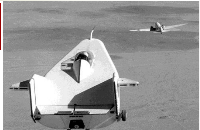
C-47 Towing the M2-F-1 to 12, 000 Feet for launch.
