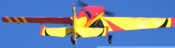
In this shot, Dane O'Brien's Extra shows the left aileron full up caught in a perfect 90 degree angle during a rolling harrier. The ailerons are at full deflection, the elevator is full down and the rudder is coming back to neutral. Dane is a great pilot
