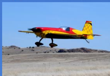
Dane's plane is a 41% Krill Extra 330SC with a 122" span. Engine is a DA170. Servos are Savox. All we can say is WOW great plane and great flying Dane!!
