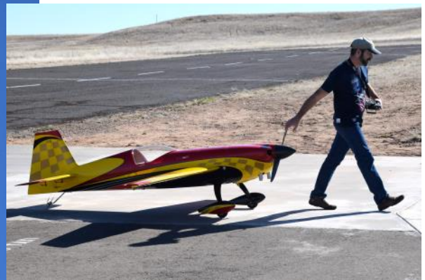
Dane's plane is a 41% Krill Extra 330SC with a 122" span. Engine is a DA170. Servos are Savox. All we can say is WOW great plane and great flying Dane!!
