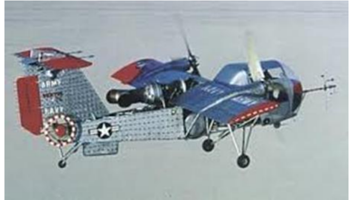
Besides demonstrating the feasibility of the tilt-wing concept, the VZ-2 program resulted in some significant contributions to tilt-wing technology.
