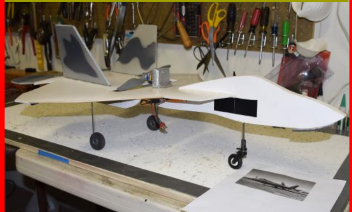
Your editor's EP foam board F-22 Raptor now has wheels, it was hand launched, landing gear will make flying it easier. Center mounted prop made it difficult to hand launch safely.
