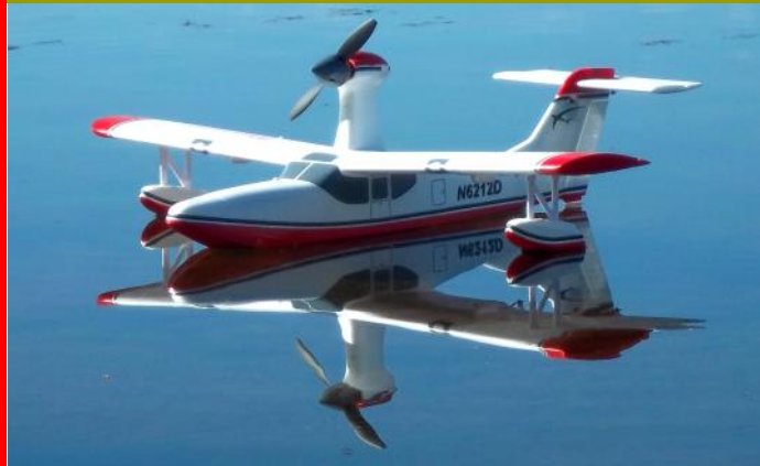
Rick Nichols' Tidewater 2 is a Flyzone RTF airplane, WS 41.5 " power is from 2200 mAh LiPo battery.
