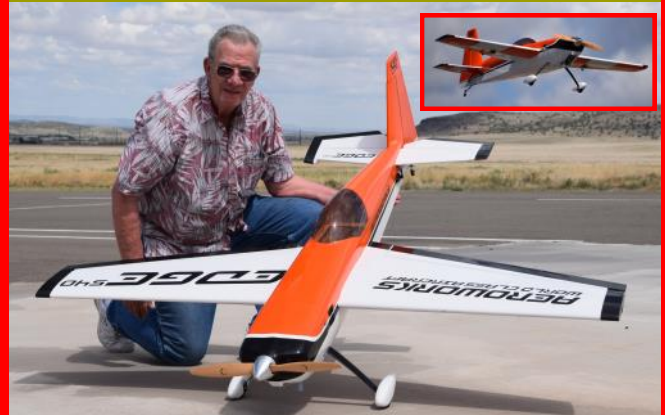
Dick Bjork's new AeroWorks Edge 540 QB ARF: Wing Span - 74"; Fuselage is 70" long. The plane's weight is approximately 10.5 pounds without gas.
