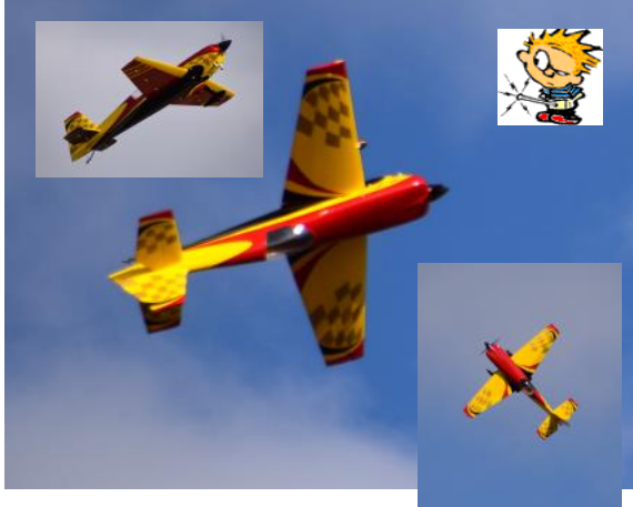
Dane O'Brien's plane is a 41% Krill Extra 330SC. Power is from a gas DA 170 and using Savox servos with a Power Box flight computer. Radio is a JR12X.
