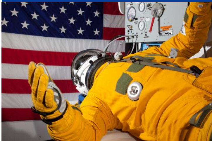
A U-2 pilot in a special pressurized space suit designed for the U-2.
