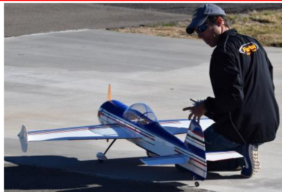
Don Crowe and his "Honda" It's a Sukhoi 60" SU-26M with a cobra motor and a 6 cell 4250 mAh battery for power.
