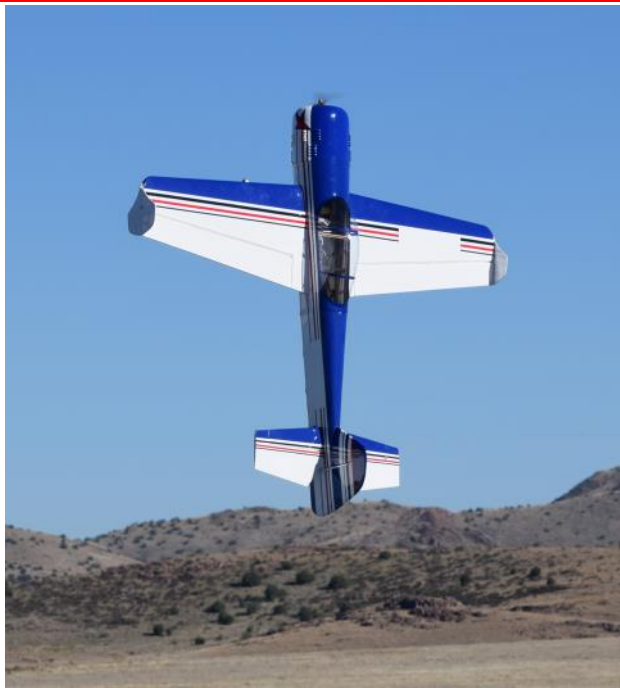
Don Crowe and his "Honda" It's a Sukhoi 60" SU-26M with a cobra motor and a 6 cell 4250 mAh battery for power.
