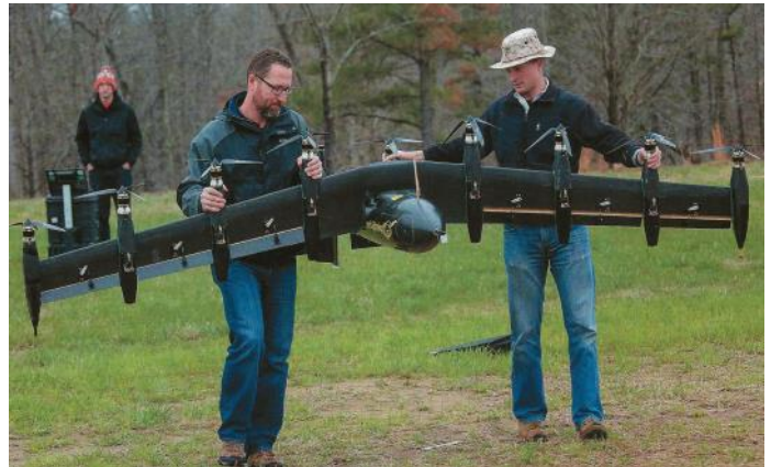
Nasa engineers prepare their large scale model for flight. The model was successfully flown on a tether indicating flight stability for the go ahead for a full scale prototype.
