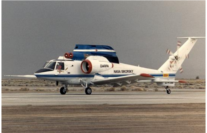
NASA high speed taxi test of the Sikorsky S-72 "X" Wing in 1987. The earlier S-72 helicopter did fly in 1976 see picture in article at left. This was before the "X" wing concept design.
