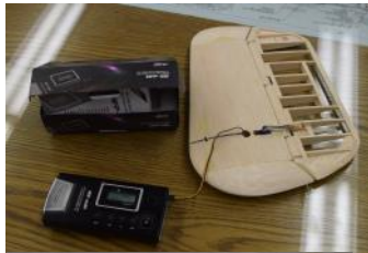
Dennis O'Connor's digital servo programmer for his vertical stabilizer.
