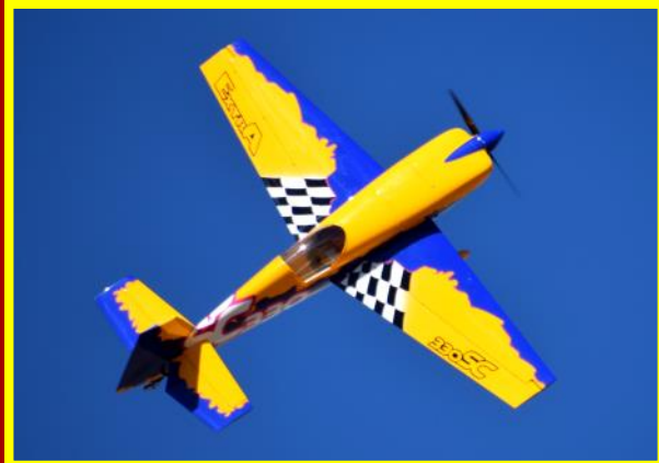
Dane O'Brien's Krill 31% Extra 330 powered by a DA70 twin with Savox servos for flight control surfaces.
