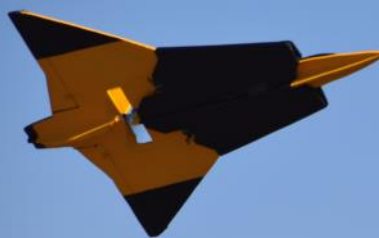
Shel Leibach launches his foam pusher Draken made by Jack Allen from plans, power is from a Hobby King 2826 2200KV motor with 6x4 pusher prop and a 3s 1600 battery.
