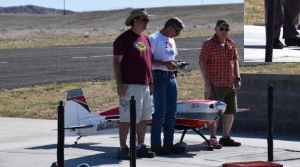
Chuck Hebestreit (above) checks engine on his 42% Edge 540 while Don Crowe and Charlie Gates assist. Chuck's 100' WS plane weights 50 lbs. with a BCC 204CC twin.
