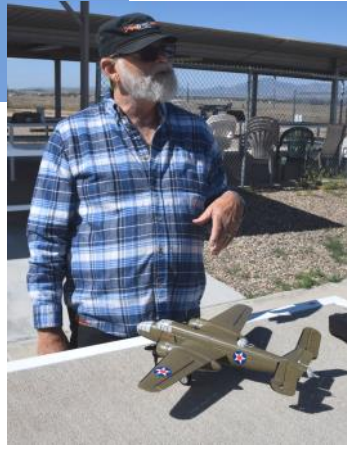
Dale Tomlinson's wee electric B-25; it has a 24" wing span - powered by a one cell 300 mah battery.
