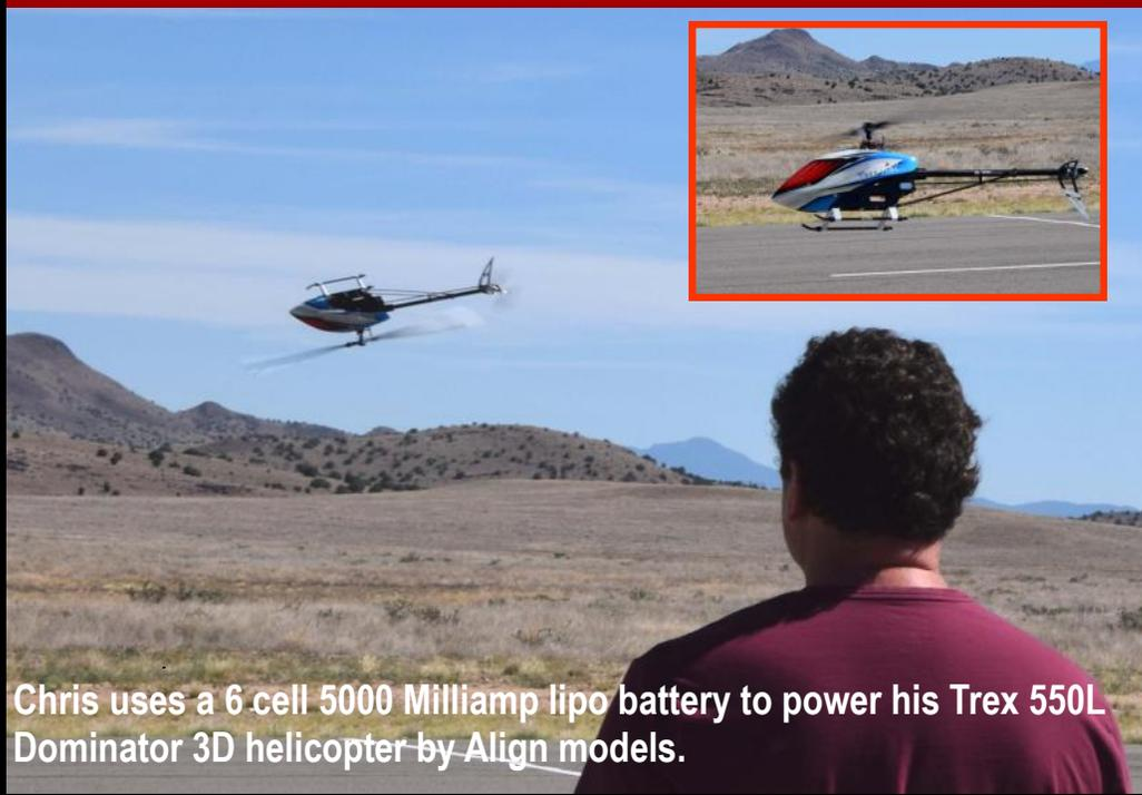
Chris uses a 6 cell 5000 Milliamp lipo battery to power his Trex 550L Dominator 3D helicopter by Align models.
