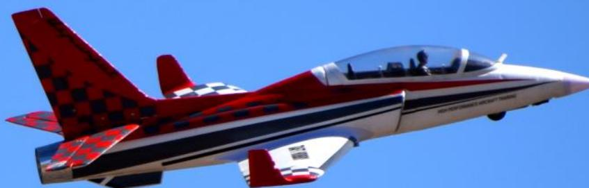
This Hobby "Viper" is powered by a 55" 90MM electric ducted fan (EDF) with a 80Amp ESC. Shel uses a 6 cell 5000 Milliamp lipo battery.
