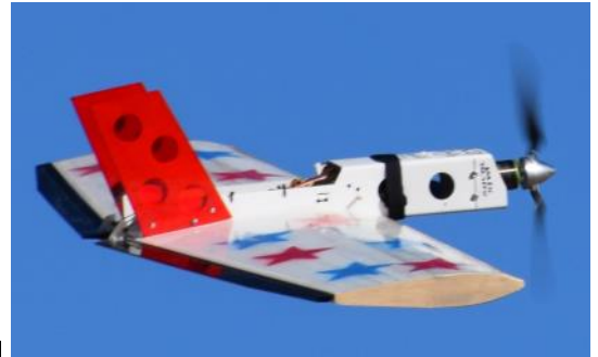
Marc Robbins flying wing, fuselage is a drain pipe, wing is foam. A great flyer.
