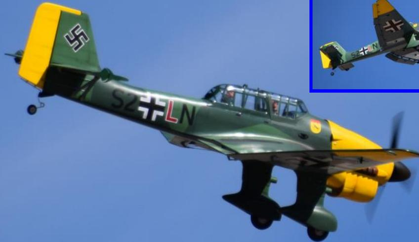
This Stuka is a 75" ARF from *Phoenix Models*. Dennis says it was one of the best ARF's out there. It took him 20 hours to finish. Dennis weathered the authentic finish then sprayed it with clear matte. Phoenix Models also installed all the hardware, Flaps, Ailerons and DLE20 engine.
