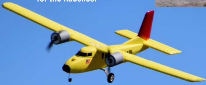
Larry Parker's very nice foam electric twin, he used prescription pill bottles for the nacelles.
