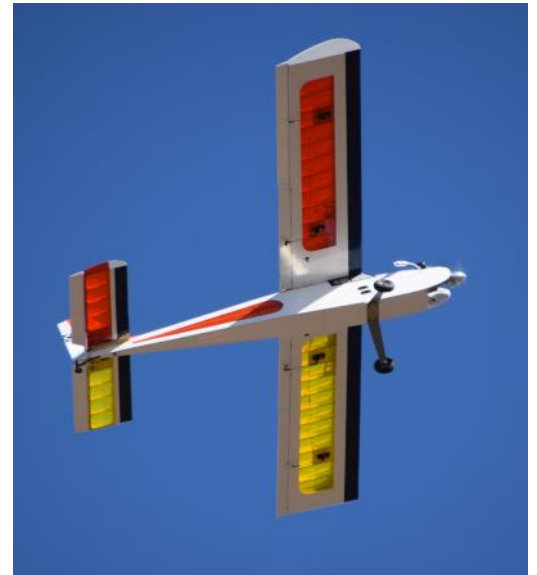
The four Telemaster wing servos for ailerons and flaps are visible in the colorful clear Monokote as she passes overhead.
