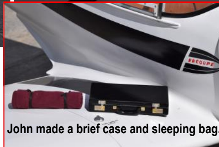
There's a lot of detail on the Ercoupe at many Internet sites. John did an outstanding job making his as scale as he wanted it. John says some he has seen have stitching and rivets. John covered the Ercoupe with Monokote. Great scale version John!
