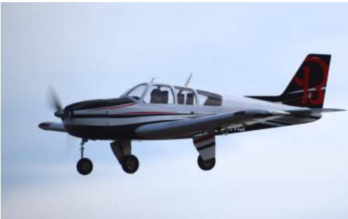
Shel Liebach's Beech Bonanza left is a VQ model and has .46 motor on 5 cell 5000. Shel's Great Planes Cirrus T22 at right has a 3600 mAh battery for power.
