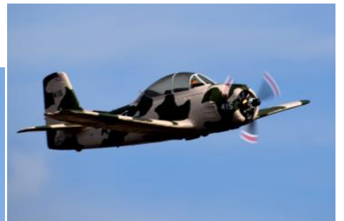
Shel Liebach also flew his T-28 above with a repainted camo scheme. It has retracts and has .25 motor with power from a 4 cell 5000 lipo battery.
