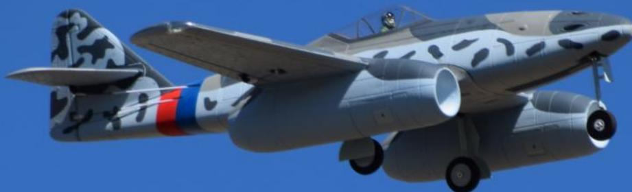
Don's Dynam ME-262 has a wing Span of 59" and is powered by two electric ducted fans with electric retracts and flaps. He uses one five cell Lipo for power. Both fan units are upgraded 70 mm units with 12 blades for more power. Weight is about 88 oz. Don also installed LED Navigation lights. He uses two 80 amp ESC's for the 2150 KV motors.
