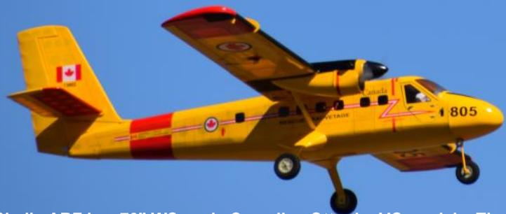
Shel's ARF is a 73" WS scale Canadian Otter by VQ models. The plane has two Tacon 25 motors with two 60 amp ESC. He uses two 4 cell 3600 milliamp batteries to power his Otter, it flies very scale-like.
