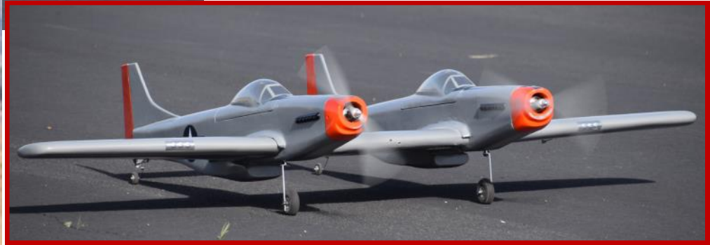
Don Ferguson test taxied his cool electric twin Mustang. His test taxi uncovered the fact his plane needs more power for our altitude so he is planning to install bigger motors and a larger LiPo battery for more power.
