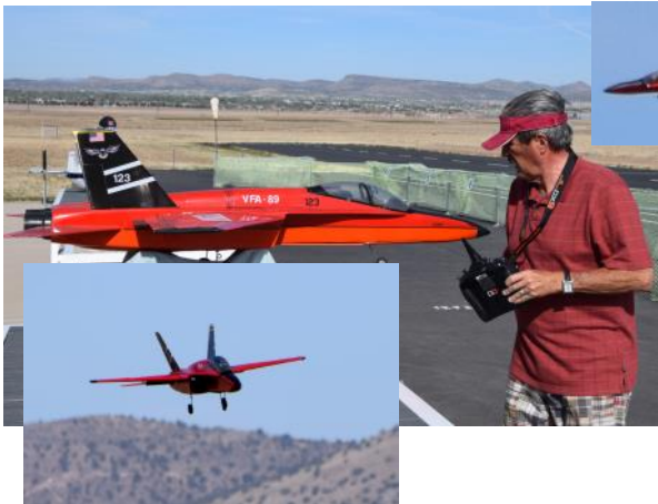
Shel Liebach and his all balsa F-18 EDF in bright orange. He uses two huge LiPo batteries to power two EDF motors.
