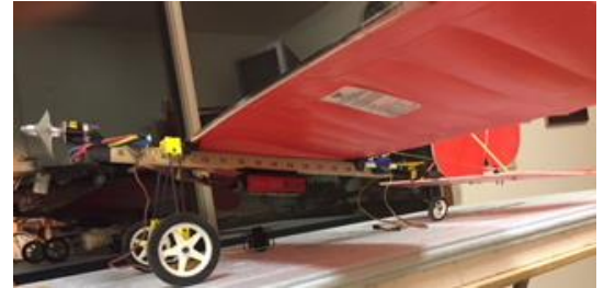
Rick Nichols' yard stick fuselage repaired slow stick.
