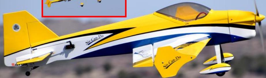
This is a balsa and ply Tower Hobbies RC model. The wing is light weight and is one-piece dual tapered with Side Force Generators increasing airflow over the ailerons stabilizing the aircraft in flight. These can be removed. Model is covered in MonoKote and has a fiberglass cowl and aluminum landing gear.
