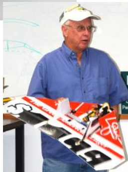
Jack Potter's Delta wing made from sign material, a good inexpensive combat ship — possibly a future event?
