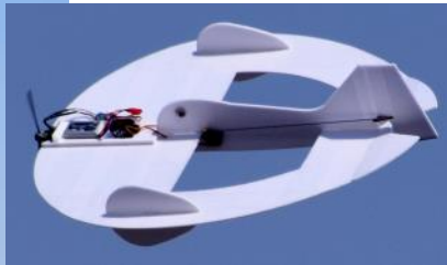
Steve Zingali's "Ground Pounder" UFO. He designed it small primarily to fly slow for indoor flying in a gymnasium.
