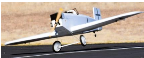
John's D-1 is powered by a four stroke .36 gasoline engine.
