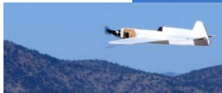
Below Rick Nichols launches Randy Meathrell's C/L Nobler at right. The battery and flight gear is on the outside along with a small wing tip weight to keep the lines tight for flight control.
