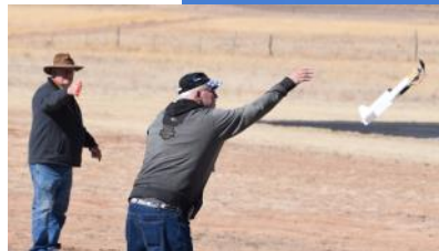
Below Rick Nichols launches Randy Meathrell's C/L Nobler at right. The battery and flight gear is on the outside along with a small wing tip weight to keep the lines tight for flight control.
