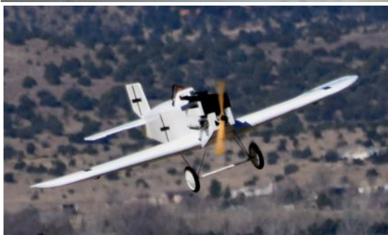
John's D-1 is powered by a four stroke .36 gasoline engine.
