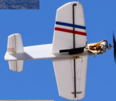
Below Rick Nichols launches Randy Meathrell's C/L Nobler at right. The battery and flight gear is on the outside along with a small wing tip weight to keep the lines tight for flight control.
