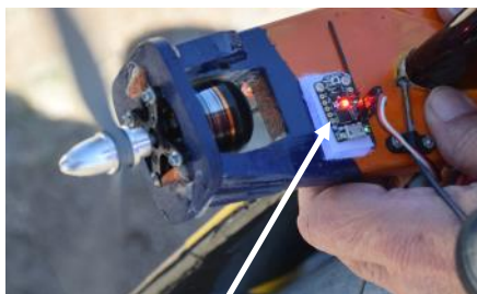
Rick Nichols' timer light indicates it's ready to fly on this test of flight time for his little C/L Ringmaster at right.
