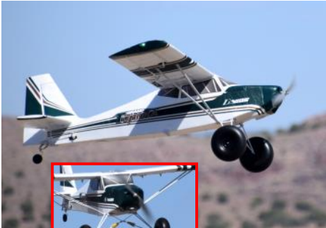
Matt Hinshaw's Cub (L) with Tundra wheels that are functional just like those used on full sized aircraft for rough field take off and landings.
