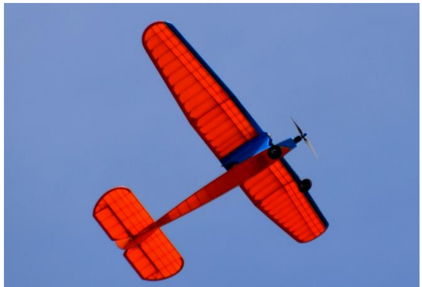
Above is Brian Jones beautiful stick and tissue-type covered glider with the sun shining through the covering. His glider was exceptionally light and was excellent in capturing thermals and gaining altitude. The glider is a 1938 balsa Leisure kit no longer made.
