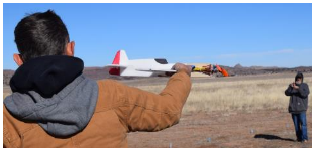
Harold Ellis helps Steve Zingali check the elevator position with the C/L handle on Steve's Nobler.
