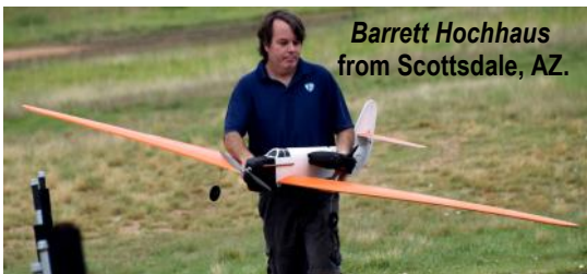
Grumman AF-2S Guardian 64-inch wingspan, Power 25 motor. 3-cell lipo power
