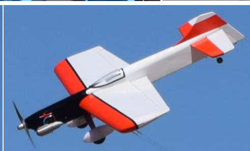
Darren Brooks at right flying his beautifully built control line Brodak Vector 40 ARC. He used medium silks span and dope an Park Lite film on the wings and tail to keep it light It's powered by an OS40.
