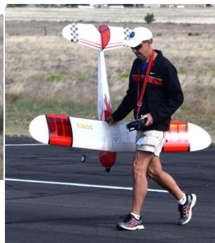
Darren Brooks at right flying his beautifully built control line Brodak Vector 40 ARC. He used medium silks span and dope an Park Lite film on the wings and tail to keep it light It's powered by an OS40.
