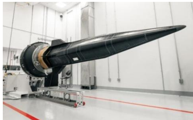
The Australian hypersonic Dart is three meters long, is hydrogen-powered and designed for testing high-temperature alloys using scramjet technologies .
